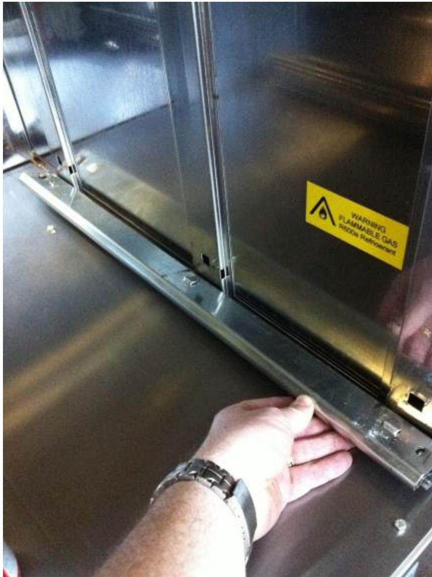
*Figure 19c: Fixings in vertical wall supports and lancing's in runner outer beam*
