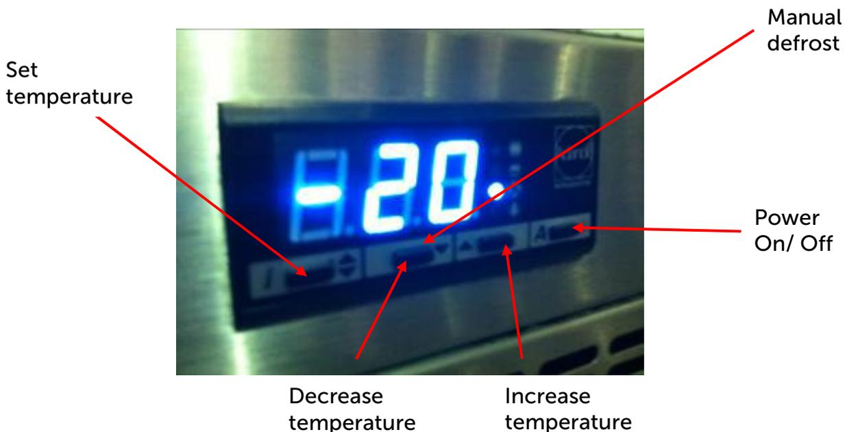
*Figure 2: Adande® Display Control Panel*
