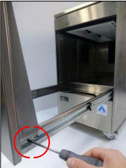
*Figure 9: Removing the two screws*
