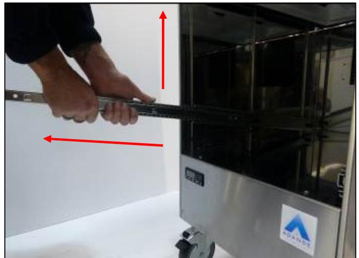
*Figure 19b: Lift and pull forward*
