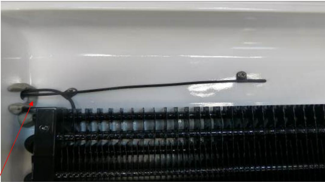
*Figure 17: Temperature probes held in place with P-Clips*
